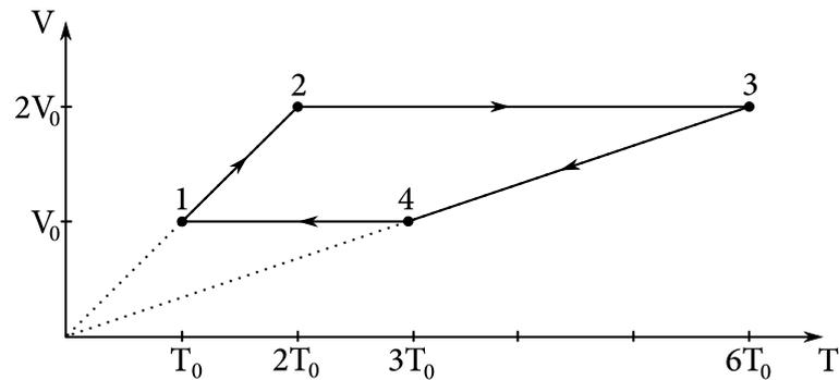
Figura 14: Cycle redrawn to VT diagram
