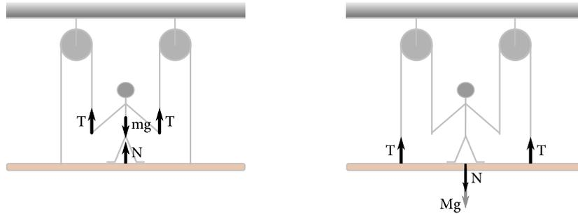
Figura 13: *Left: forces acting on the strongman. Right: Forces acting on the board*
