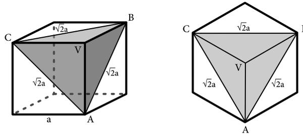
Figura 18: *A cube inclined to the Sun with the greatest possible surface*
