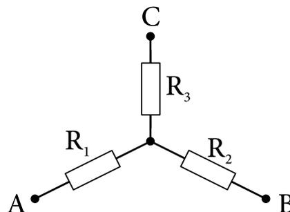
Figura 1: Resistors connected into the shape of a star
