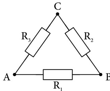
Figura 2: Resistors connected into the shape of a triangle
